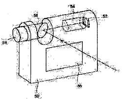
54. The prism 56 is rotated by a prism rotating knob 58 with reference to the main body 50, thus, the photographing direction is continuously changed at an angle ≥ almost 180° in a plane vertical to the optical axis of the photographic lens 54.
